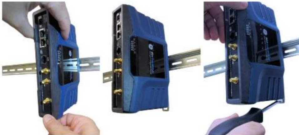
Figure 2-9. DIN Rail Attachment and Removal (Pull down tab to release from rail)
