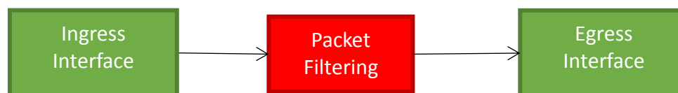
Figure 3-122. Packets Being Forwarded Through the Unit
