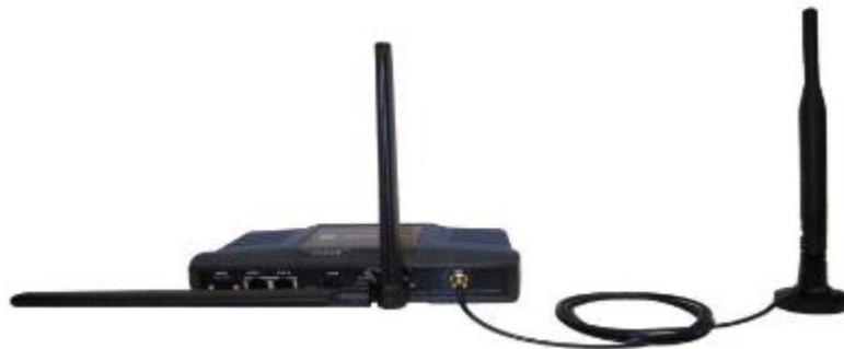
Figure 2-11. Direct Mounting of Cell Antenna; Cabled WiFi Antenna Minimum 8-inch (20.32 cm) separation between cell and WiFi antennas
